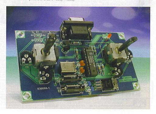
FMS encoder. Where these connections are will depend on what type of R/C you have. A few are listed in **Figure 3**. You may have more information available from your radio control manual. If you are unsure which connections to use then don't be afraid to experiment since the buffered input is quite safe. If you fail to place them the right way around the encoder will behave erratically — just swap them over and everything should be okay.
